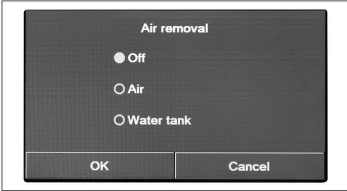
After opening the "Air removal" function, user can activate (inside the selected circuit) water circulation to bleed any air in the circuit. Once the required logic has been selected, press "OK" to confirm.
