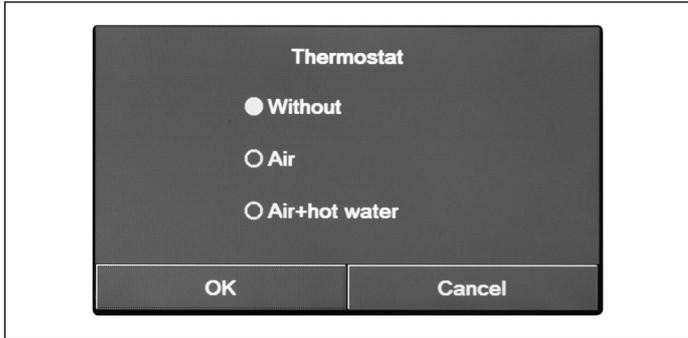
After opening the "Thermostat" function, user can specify which management type can be applied to any external thermostat. Once the required item has been selected, press "OK" to confirm.
