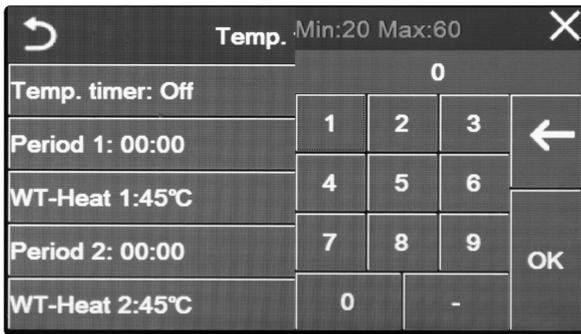
Click the labels concerning the parameters of flow temperature and a numerical keypad will be displayed on the right-hand side (together with the permitted range Flow temperature), which allows user to enter the required values.
